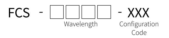
For example, FCS-0470-000 is a 470nm fiber-coupled light source with SMA fiber adaptor.
